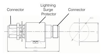
To ground your surge protector, use 10 or 12-gauge copper wire and attach it to the ground connector screw. Tighten the screw so the wire is firmly embedded under the screw. Next, clip the other end of the wire and strip back the jacket to expose the raw wire. Then, attach the wire to a grounding point or rod sunk into the ground 8 feet deep. Be sure to check your local grounding code requirements as they vary by location.
